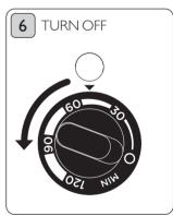
If you need to turn the oven off before the timer has finished, set the function dial to 'OFF' and turn the timer to '0'. You will hear the bell.
